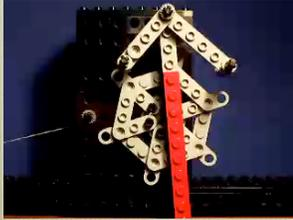
Escapement: must transfer energy to pendulum to keep it swinging
