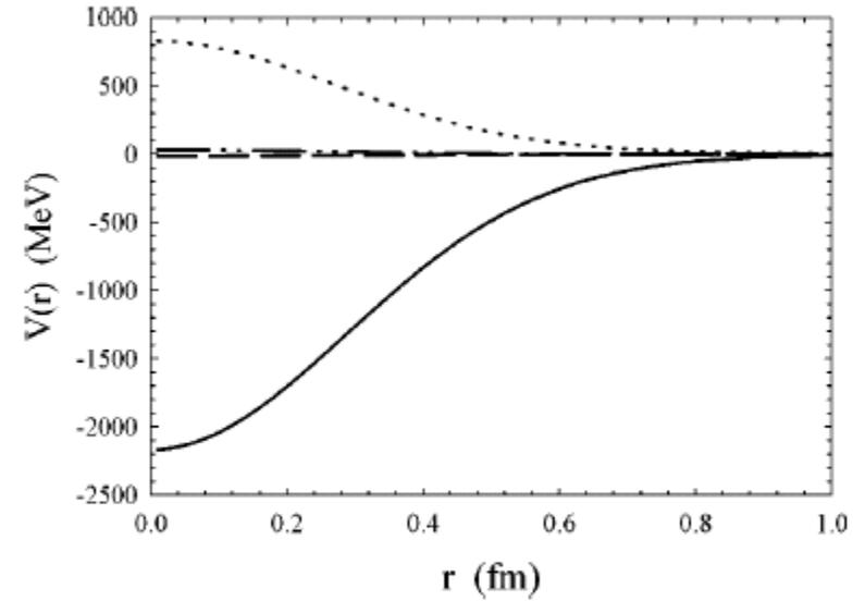
FIG. 2. The  $\pi\pi$  potentials vs  $r$  for  $I=0, L=0$  (solid line),  $I=0, L=2$  (dashed line),  $I=2, L=0$  (dotted line), and  $I=2, L=2$  (dot-dot-dashed line). The potentials are given by Eq. (8) with the
