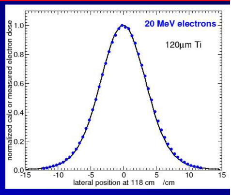
Note the experiment is slightly wider than calculations
