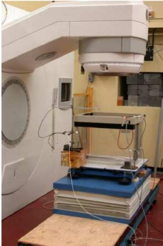
Figure 2.2: Phantom setup for a dosimetry measurements in water with the Scanditronix water phantom tank and dosimetry scanner
