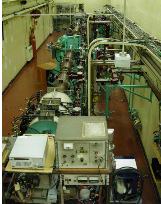
Figure 3.1: The NRC Vickers research linac. Electrons are accelerated towards the far end. From the NRC-IRS website, with permission.
