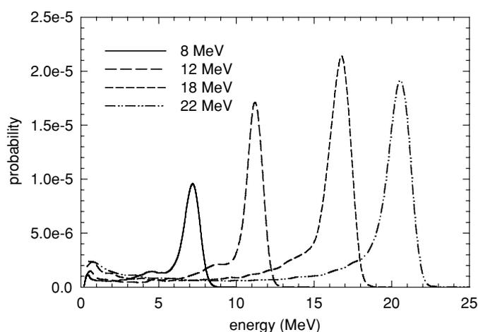
**Figure 4.** Spectra at the central axis of 8, 12, 18, 22 MeV electron beams from the Elekta precise medical linac generated by BEAM Monte Carlo code (Rogers *et al* 1995). Field size 10 cm  $\times$  10 cm on the phantom surface with SSD 100 cm.
