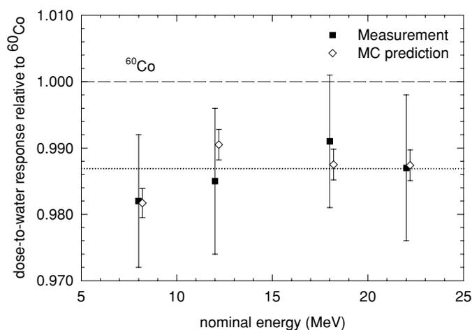
**Figure 5.** A comparison of measured and Monte Carlo calculated values of the alanine response per unit absorbed dose-to-water for electrons relative to that of  $^{60}\text{Co}$ . The measurement data are corrected for the effect of the dosimeter holder. The dotted line drawn at 0.987 on the y-axis indicates the average lower response of 1.3% for electrons relative to  $^{60}\text{Co}$ . Note that the error bars on the Monte Carlo calculations are statistical only.
