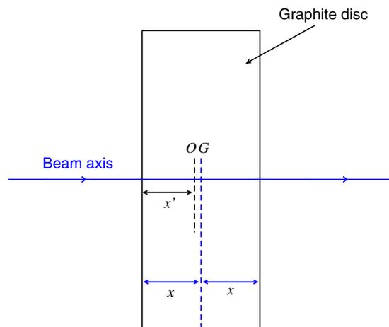
**Figure A1.** The factor  $\tilde{t}_c$  (equation (A.5)) calculated for the experiment of Guiho and Simoen relates the dose to a graphite disc centred at  $G$  to the air kerma at a point  $O$ , a distance  $x-x'$  upstream from  $G$ . The distances indicated are  $x = 0.55$  cm ( $0.940$  g cm $^{-2}$ ) and  $x' = 0.49$  cm ( $0.83$  g cm $^{-2}$ ). The centre of the graphite disc,  $G$ , is  $100$  cm from the  $^{60}\text{Co}$  source.
