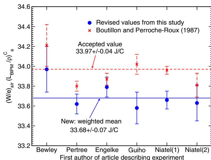
**Figure 1.** Values of  $(W/e)_{\text{air}}(\bar{L}_{\text{BIPM}}/\rho)_a^C$  reported by Boutillon and Perroche-Roux (1987) and from the current analysis. The accepted value, based on the results of 15 experiments (Boutillon and Perroche-Roux 1987) and the uncertainty of 0.11% recommended by the CCRI (1999), and the weighted mean for the updated results are indicated.
