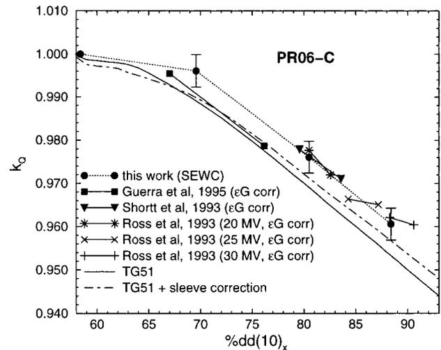
FIG. 7. Same as Fig. 6 but as a function of  $\%dd(10)_x$ . The full line and the dashed-dotted line show the data from the TG-51 protocol (Ref. 4) and the data from the TG-51 protocol with correction for a 1 mm PMMA sleeve, respectively. SEWC stands for sealed water calorimeter.
