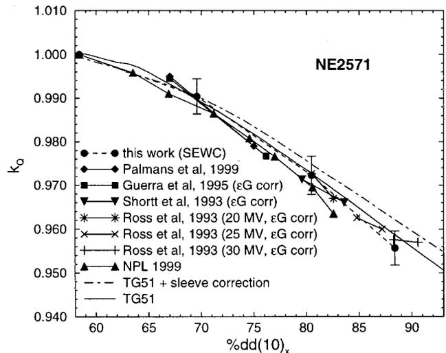
FIG. 3. Same as Fig. 2 but as a function of %dd(10)<sub>x</sub>. The full line and the dashed-dotted line show the data from the TG-51 protocol (Ref. 4) and the data from the TG-51 protocol with correction for a 1 mm PMMA sleeve, respectively. SEWC stands for sealed water calorimeter.
