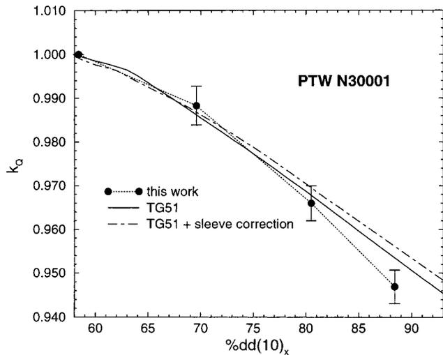
FIG. 8. Measured beam quality correction factors  $k_Q$  for the PTW-N30001 chamber as a function of  $\%dd(10)_x$ . The full line and the dashed-dotted line show the data from the TG-51 protocol (Ref. 4) and the data from the TG-51 protocol with correction for a 1 mm PMMA sleeve, respectively.
