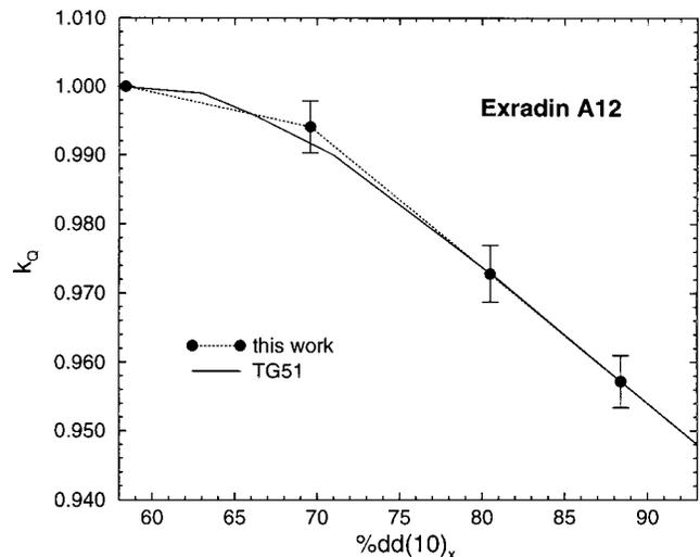
FIG. 9. Measured beam quality correction factors  $k_Q$  for the Exradin A12 chamber as a function of  $\%dd(10)_x$ . The full line is the TG-51 values.
