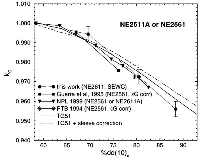
FIG. 5. Same as Fig. 4 but as a function of  $\%dd(10)_x$ . The full line and the dashed-dotted line show the data from the TG-51 protocol (Ref. 4) and the data from the TG-51 protocol with correction for a 1 mm PMMA sleeve, respectively. SEWC stands for sealed water calorimeter. Values of  $\%dd(10)_x$  for other PTB beams in Fig. 4 were not available to us (see text).
