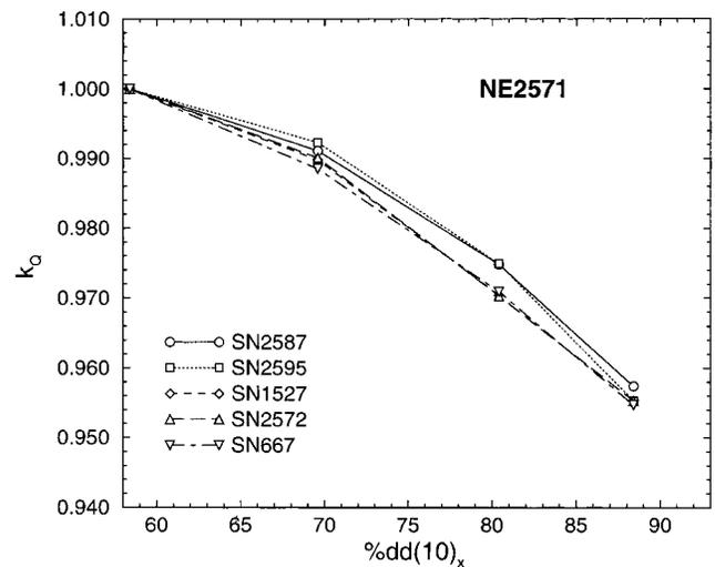
FIG. 1. Absorbed dose beam quality conversion factor  $k_Q$  for five chambers of the NE2571 type as a function of  $\%dd(10)_x$ .
