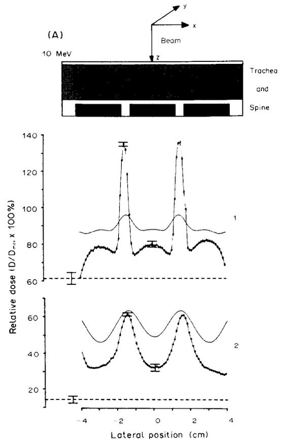
Fig. 6. Lateral dose profiles in water, 0.1 and 1.1 cm behind a phantom with a 2.6 cm dia rod of air and 3 aluminum disks (2.5 cm dia, 1 cm thick) embedded in wax and separated by 0.5 cm. Beam energy was 10 MeV. From Cygler *et al.* (1987).
