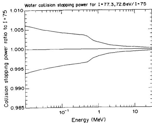
Fig. 2. Ratio of water collision stopping powers calculated with  $I$  values of 77.3 and 72.8 eV ( $2\sigma$  limits on the experimental values of  $I$ ) to those calculated with the ICRU Report 37 recommended  $I$  value of 75 eV.
