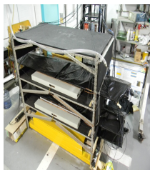
Fig. 4 Test muon detector (1x1 m 2 ) in Carleton is currently taking data shown in Fig. 5.
