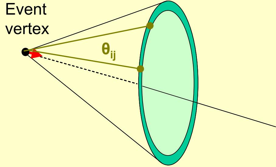
Isotropy variable,  $\beta_{14}$ , function of angles between each pair of hit PMTs ( $\theta_{ij}$ ) in event
